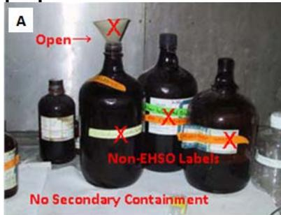
The waste is NOT properly labeled, segregated by compatibility, closed or stored in secondary containment.
