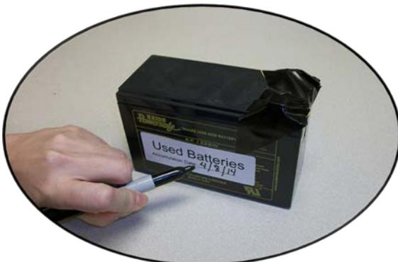
Label: "Used Batteries" and Date Removed from Service
