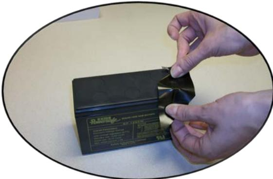
Cover Electrodes with Non-Conductive Tape without Covering Labels
