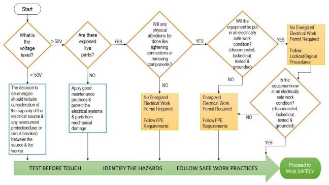
Source: From Figure J.2 (NFPA 70E Standard for Electrical Safety in the Workplaces, 2018
